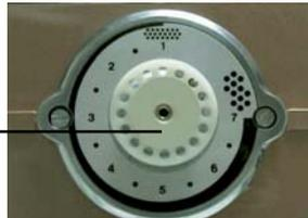
4. If you grind some beans now, you should get fine grains. If the coffee beans have been ground too fine, the discs can stick together. The grinder would be blocked.
